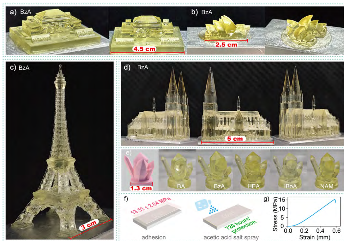
Figure 3. a–d) 3D-printed world landmark replicas fabricated using the BzA-based resin. e) Models printed using different resins. f) Schematic illustration of the anticorrosion coating strategy based on DTI-mediated photoiniferter polymerization, highlighting coating adhesion and salt spray resistance performance on Q235 steel. g) Stress–strain curve from the pull-out test of the photo-cured coating.
